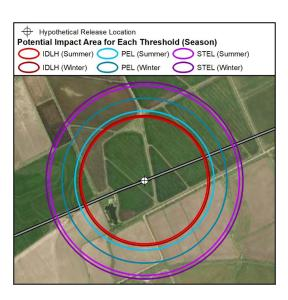
A diagram of the distances of various threshold levels of a hypothetical release with concentration levels at multiple distances
